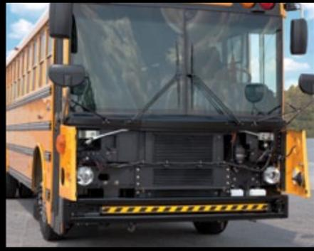
Routine maintenance is easy on the EFX. The front access panel provides quick access to wipers, as well as the heater core and filter. And the design helps reduce noise inside the cabin.
