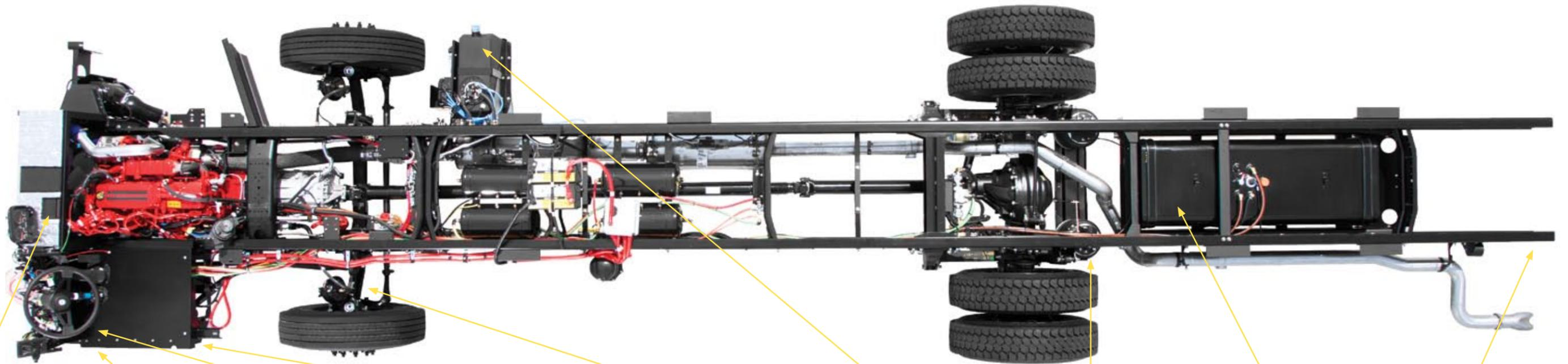
Easy access to power steering reservoir, wiper motors, and washer fluid for easier serviceability
