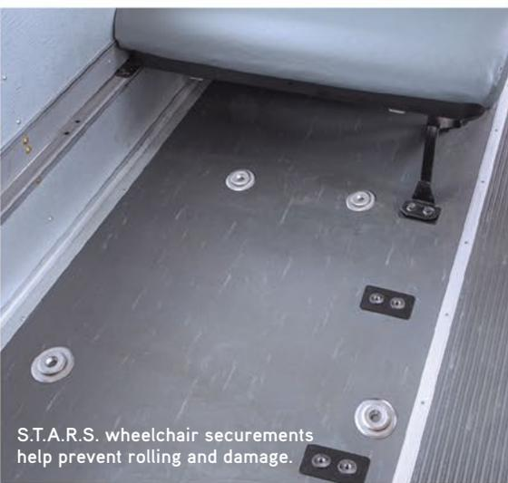
S.T.A.R.S. wheelchair securements help prevent rolling and damage.
