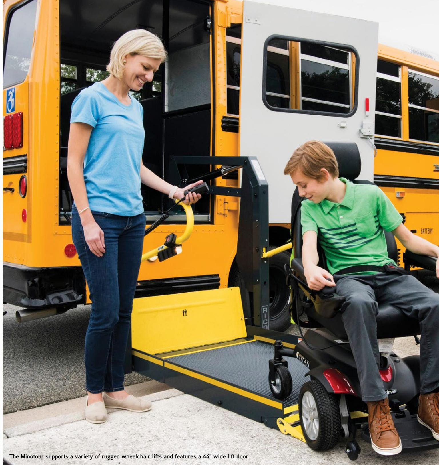
The Minotour supports a variety of rugged wheelchair lifts and features a 44" wide lift door
